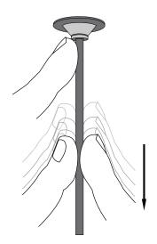
The length of the cable is adjustable. To determine the proper length of the fixture, hold the fixture canopy up against the outlet box in the ceiling to adjust the cable.
