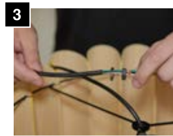
Pass lock washer and nut through cable.
