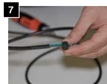
Feed additional strain relief through cord.
