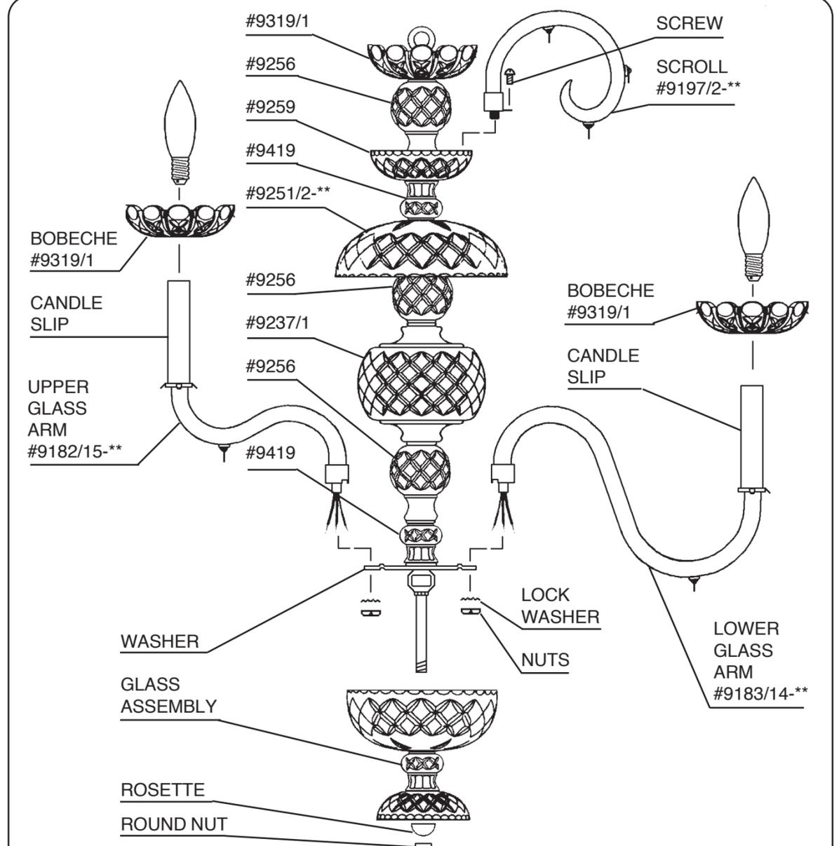
**8** Install scrolls into washer with screws provided. Install arms into large arm washer. Line up holes in arms with dimple in washer. Use lock washer and nut to secure arms in place. **NOTE: 5 Upper arms into inside diameter holes and 10 lower arms into outside diameter holes.**
