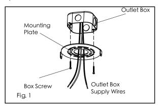
2. Pull wall box wires through center hole of mounting plate. Secure mounting plate to wall using screws so that the fixture mounting points are aligned vertically. (See Fig. 1)
