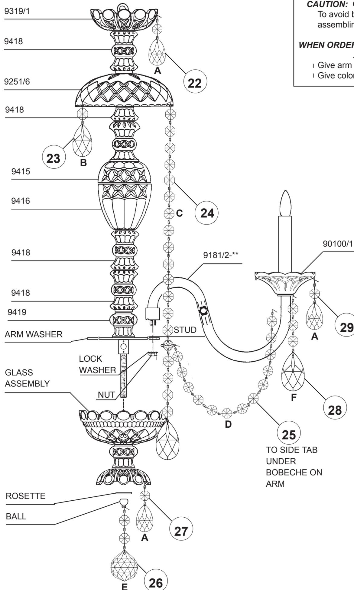
**CAUTION:** Glass parts are fragile. To avoid breakage use care when assembling or cleaning.
