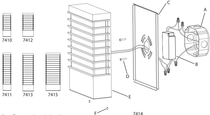
1. Shut off power to the outlet box (A).
