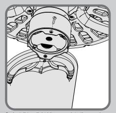
Preinstall two light kit screws into the cap ring using any two opposing holes. It does not matter which two you choose.
