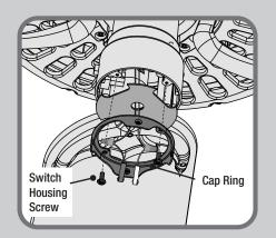
Insert the insulator back into the switch housing while passing the wires from the fan through the center hole. Lift the cap ring and align the holes with the switch housing screw holes. Attach cap ring to switch housing with switch housing screws.
