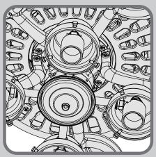
Install the final light kit screws in the remaining holes. Tighten all four screws securely.
