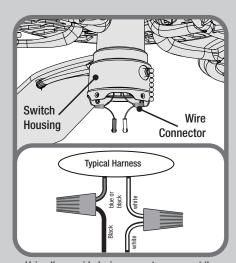
Using the provided wire connectors connect the white wire from the fan to the white wire from the wire harness and connect the black or blue wire from the fan to the black wire from the wire harness.
