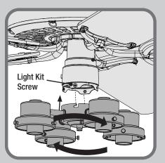
Align the notches in the sides of the light kit assembly with the screws on the upper switch housing. Twist the light kit assembly clockwise to lock into place.
