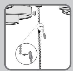
Installing the Pull chain pendant - Attach the pull chain pendant to the end of the short chains coming from the light kit.
