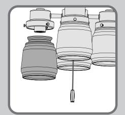
To install the shade, first loosen the thumb screws. Raise the shade to the light fixture. Tighten all thumbscrews securely.
