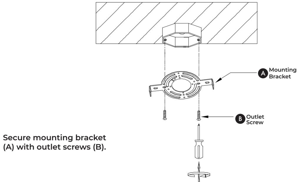
Secure mounting bracket (A) with outlet screws (B).
