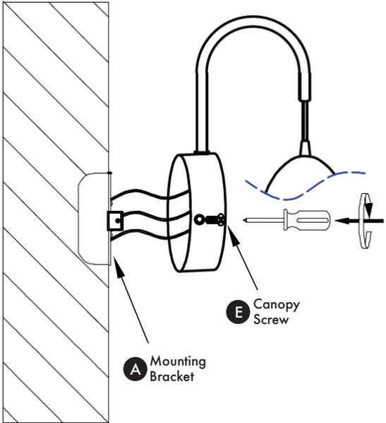
Secure canopy to mounting bracket (A) with canopy screws (E).
