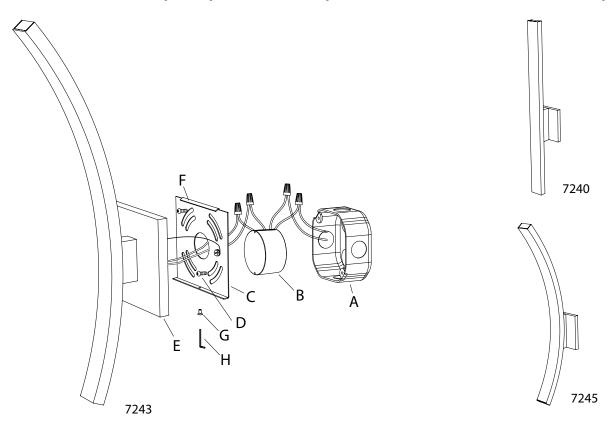
1. Shut off power to the outlet box (A).
