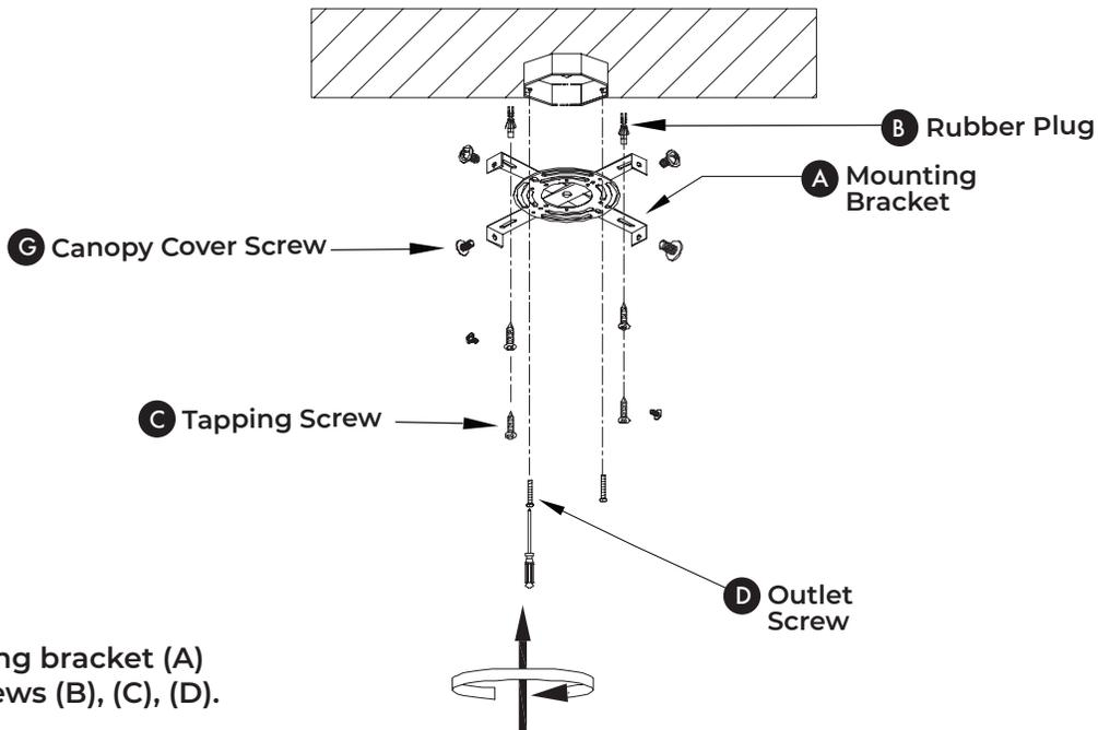
Secure mounting bracket (A) with outlet screws (B), (C), (D).
