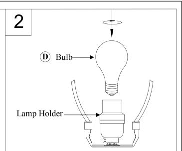
Screw on the bulb (D) make sure this is done with the power off.
