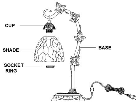
Recommended (1) maximum 60 WATT Type "A" Bulbs Or (1) maximum 13WATT CFL Bulbs (Bulbs not included)
