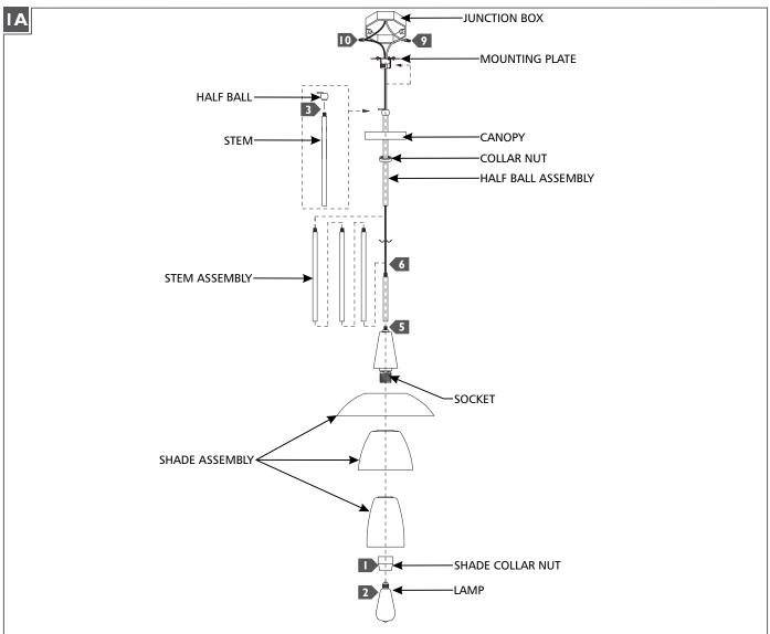
Place the shade assembly onto the socket in the order shown, then secure in place by screwing the shade collar nut onto the socket.
