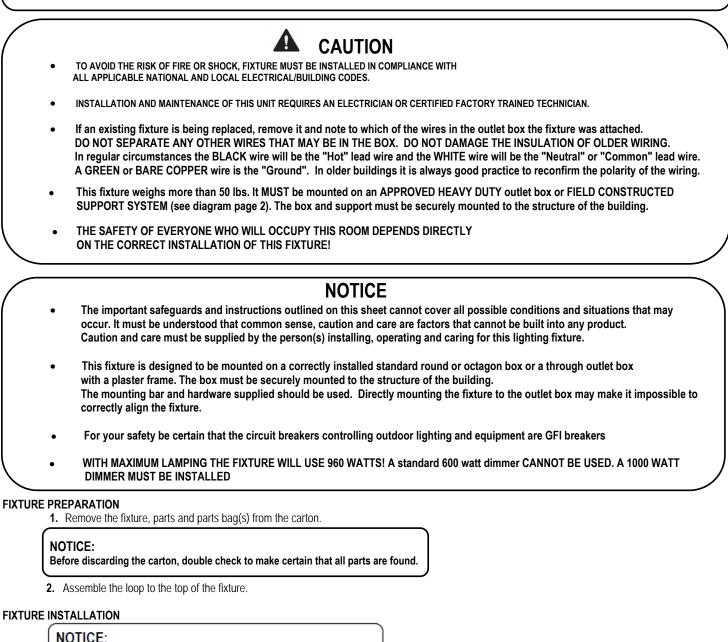
THIS LUMINAIRE MUST BE MOUNTED OR SUPPORTED INDEPENDENTLY OF AN OUTLET BOX
