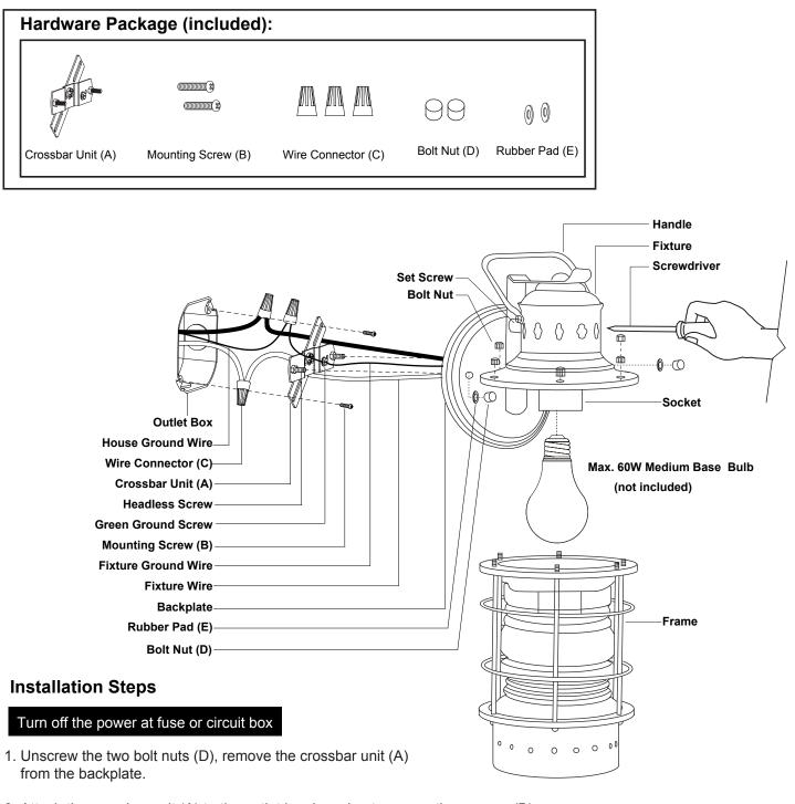
Attach the crossbar unit (A) to the outlet box by using two mounting screws (B). Adjust the length of the preinstalled headless screws if necessary. Note: Make sure that the headless screws are lined up horizontally to make the fixture level.
