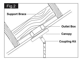
8. Angled mounting recommended for a vaulted or angled ceiling. (See Fig.2)
