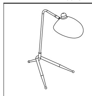
1. Insert recommended bulb (not included) into socket (A). **WARNING:** Verify correct bulb wattage marked on socket of lamp. DO NOT exceed maximum bulb wattage.
