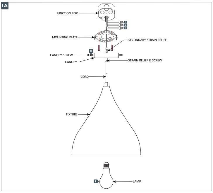
Feed the fixture cord through the strain relief and canopy until the desired height is achieved, then tighten the strain relief screw.
