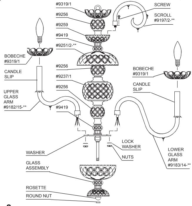
8 Install scrolls into washer with screws provided. Install arms into large arm washer. Line up holes in arms with dimple in washer. Use lock washer and nut to secure arms in place. NOTE: 5 Upper arms into inside diameter holes and 10 lower arms into outside diameter holes.
