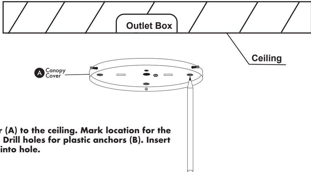
Raise canopy cover (A) to the ceiling. Mark location for the plastic anchors (B). Drill holes for plastic anchors (B). Insert plastic anchors (B) into hole.
