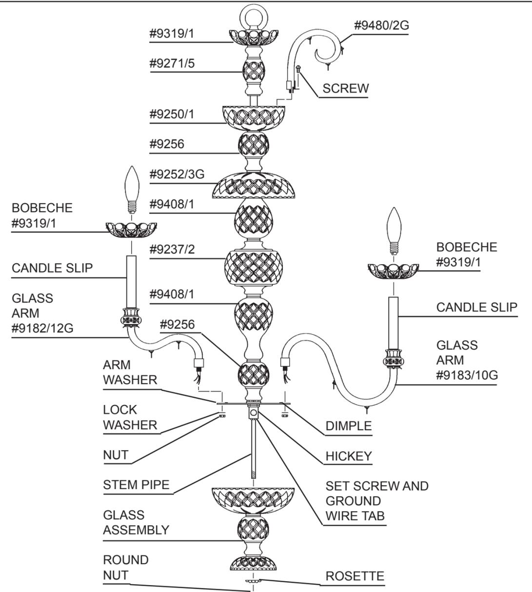
**8** Install scrolls into washer with screws provided. ALTERNATELY install two different arms into washer. Line up holes in arms with dimple in washer. Use lock washer and nut to secure arms in place.
