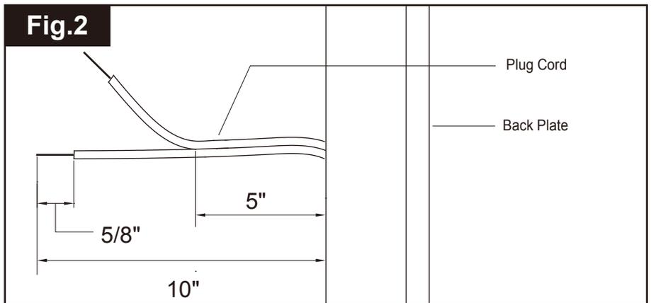
Carefully put the wires back into the backplate.
