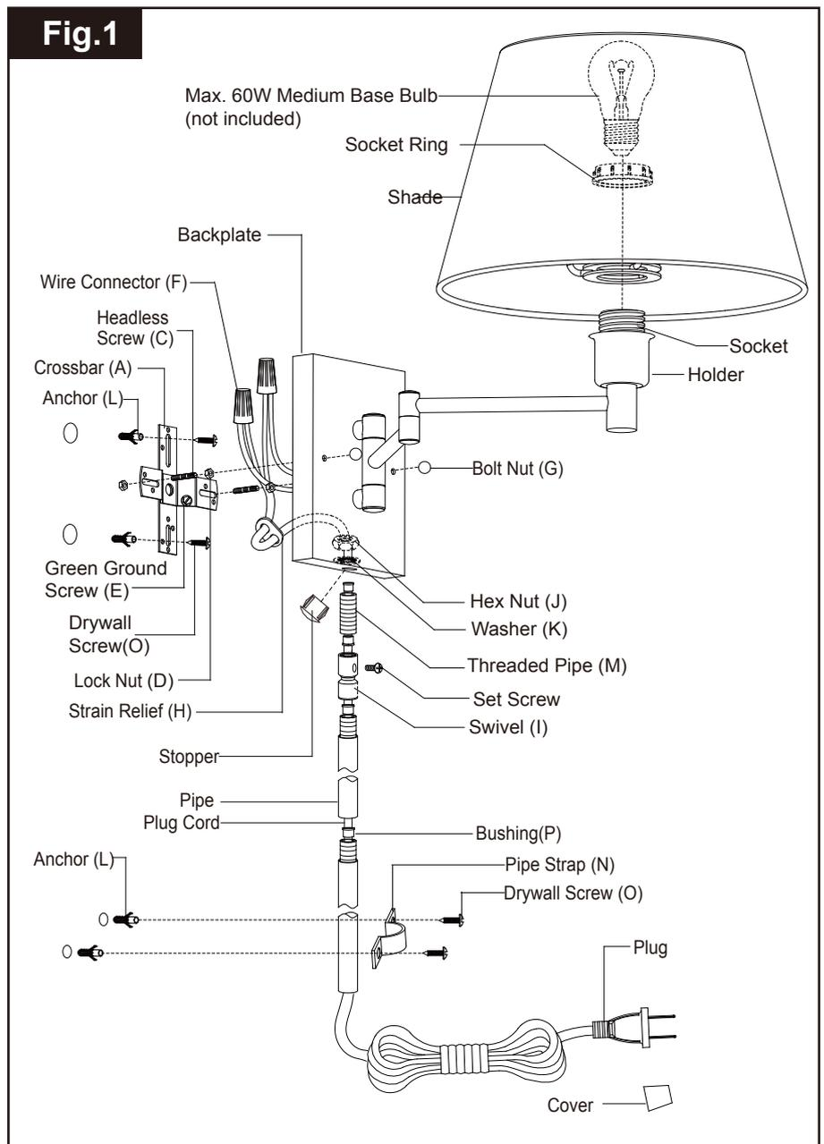
7. Thread the plug cord through two holes of the strain relief. Pull the plug cord down until the strain relief touches the backplate.
