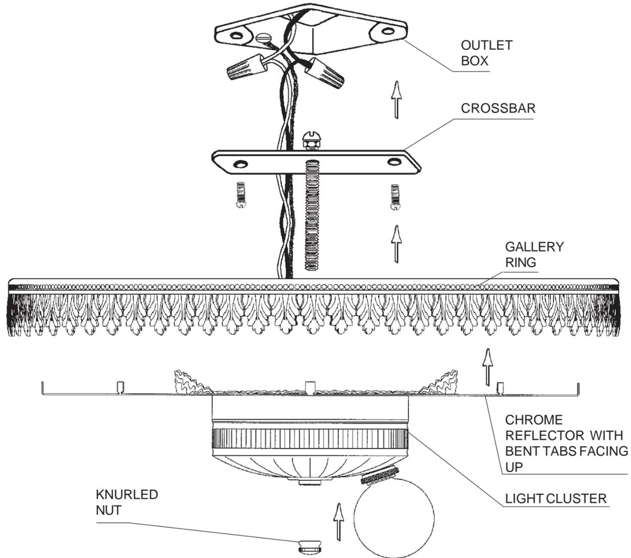
**1** Remove crossbar from light cluster and reflector. Attach to outlet box in ceiling.
