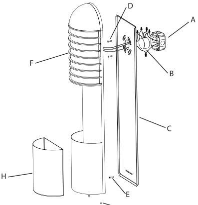
1. Shut off power to the outlet box (A).
