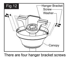
and lock washers. Remove two screws
