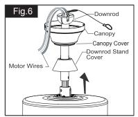
(For downrod mount only): Thread the motor wires through the downrod stand cover, canopy cover (Making sure the smooth side of canopy cover is facing downward), canopy and downrod.
