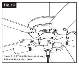
Install LED bulbs (included). See relamping label at socket area or packaging for maximum wattage allowed.
