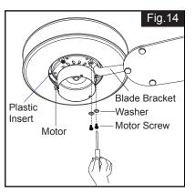
Remove the motor screws and washers from the fan motor assembly. Secure blade brackets to the motor with washers and motor screws.
