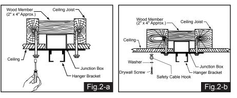
Tighten the hanger bracket to the outlet box with two mounting screws.(**Make sure the outlet box is securely installed so that it will be able to support at least the fan weight.**) Attach the safety cable hook to the ceiling with the drywall screw and washer, and make sure the safety cable hook is covered by the fan canopy. **WARNING: MOUNT ONLY TO AN OUTLET BOX MARKED "ACCEPTABLE FOR FAN SUPPORT"!**
