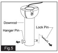
(For downrod mount only): Remove the lock pin from hanger pin and remove the hanger pin from the downrod.
