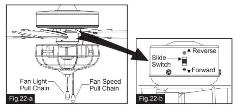
The slide switch on switch box sets direction of fan rotation. Select the desired direction of fan rotation. Push the slide switch down for "Forward" and up for "Reverse".
