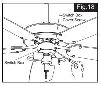
Secure the switch box cover onto switch box with the switch box cover screws.
