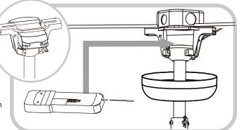
**Note:** If the electrical wire is going to be cut shorter than provided you will need to identify the label on each wire before you cut the excess wire off. Re-label the wire near where you want to make the cut. Be sure to mark the wire on the side of the fixture and not on the excess wire being cut and removed.
