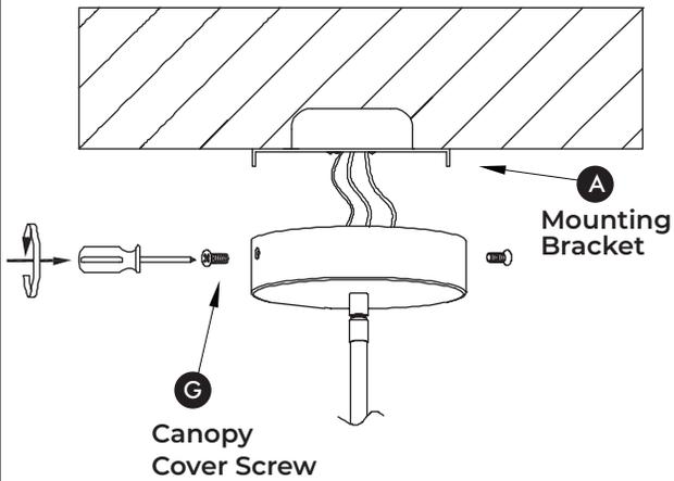
Secure canopy to mounting bracket (A) with canopy screws (G).
