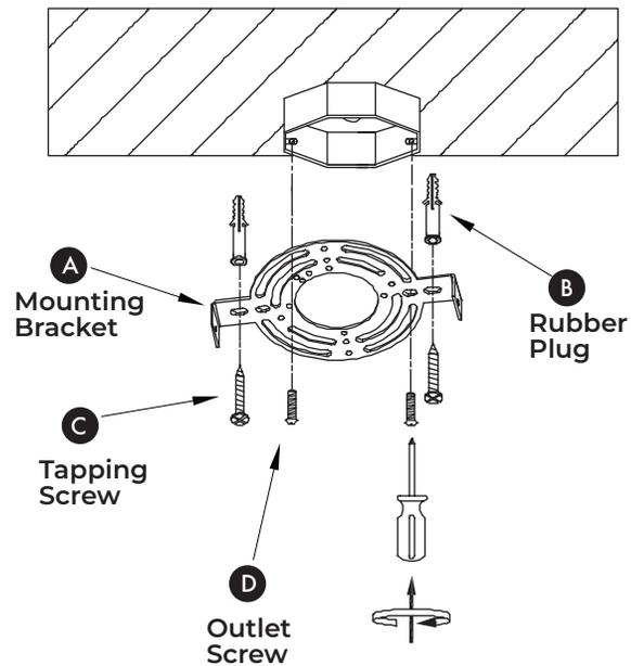
Secure mounting bracket (A) with outlet screws (B), (C), (D).
