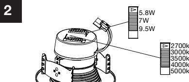
Before installation, select your preferred CCT and Wattage settings by adjusting the sliding switches.
