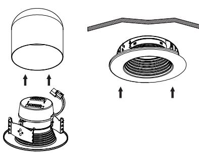
Push the LED retrofit trim into the recessed light fixture. Continue to push the LED trim until its outer edge is flush with the ceiling surface.
