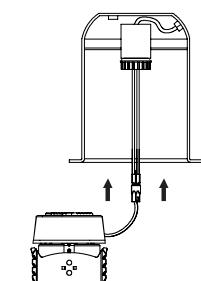
Connect the quick disconnect between the retrofit kit and the medium base umbilical socket.
