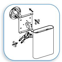
CONNECT THE WIRES AND MOUNT THE FIXTURE
