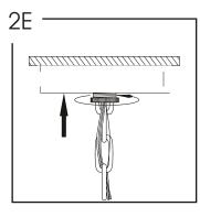
Carefully tuck wires into junction box and secure canopy to ceiling using screw collar ring.
