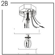
Slip screw collar ring and canopy onto chain, and hang fixture onto screw collar using an open link of chain. Close link. Thread wire and ground cable through screw collar ring, canopy, chain, screw collar, and through threaded tube on crossbar assembly. Pull wires through.
