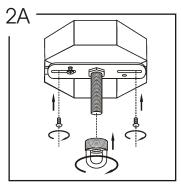
Screw crossbar assembly into junction box using outlet box screws. Thread screw collar onto threads of crossbar assembly.
