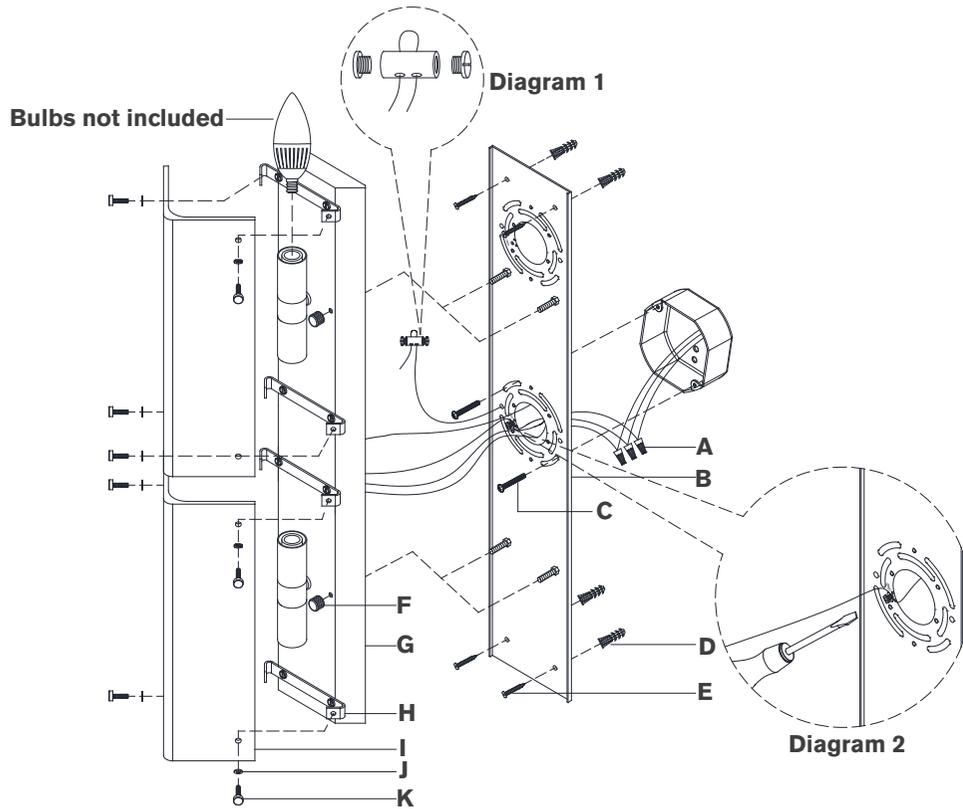
9. Connect fixture hot wire (black) to the supply hot wire (usually black) using wire nut **(A)**.
