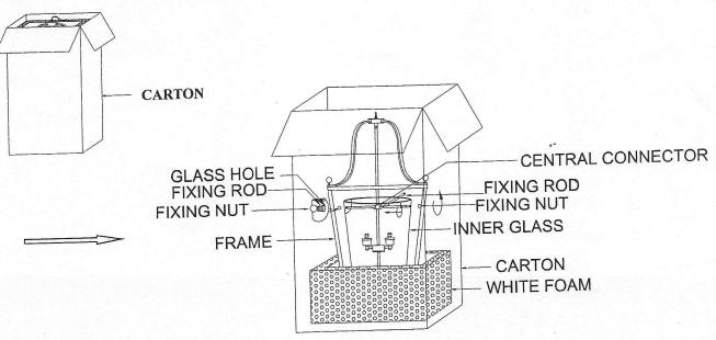
STEP 3. Install the Inner Glass to the Fixture.
