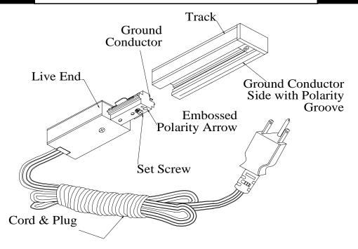
CAUTION - DO NOT plug into wall outlet until Live End is properly installed into track as shown. The contact tabs at end of Live End are "HOT" and "DANGEROUS" as soon as it is plugged into wall outles. MAXIMUM capacity Live End with cord set is 10 AMPS. DO NOT OVERLOAD.
