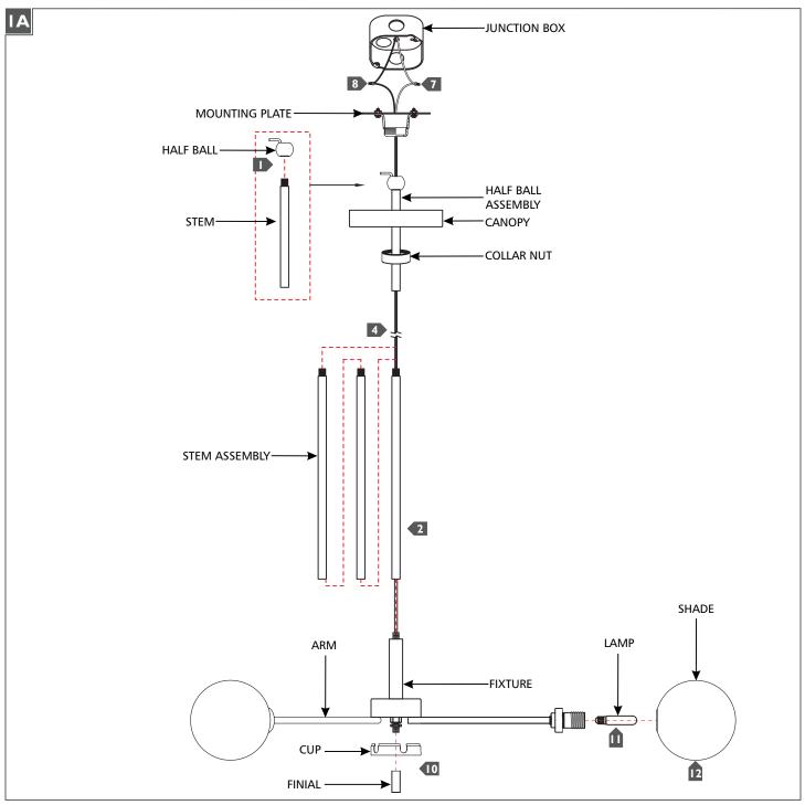
Screw the half ball to the stem which will be on top.
