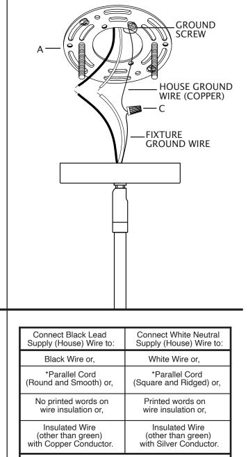
\*When parallel wire (SPT 1 & SPT 2) is used: The lead wire is round in shape or smooth. The neutral wire is square in shape or ridged.
