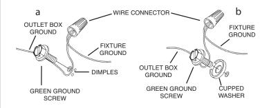
Make wire connections. Reference chart below for correct connections and wire accordingly.
