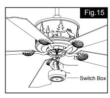
Connect the two terminals respectively from the motor and the switch box.
