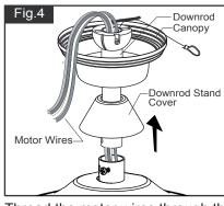
Thread the motor wires through the canopy, downrod stand cover and downrod.
