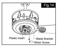
Remove the motor screws, plastic inserts and washers from fan fixture set. Secure blade brackets to the motor with washers and motor screws.
