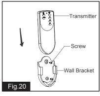
Install the transmitter wall bracket on the wall with two screws and place transmitter in it carefully.
