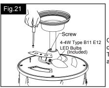
Open the inner light plate of worse bulbs by screw driver. Take off the worse bulb and install the new one.
