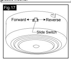
The slide switch on switch box sets direction of fan rotation. Select the desired direction of fan rotation. Push the slide switch left for "Forward" and right for "Reverse".
