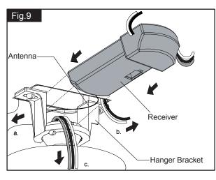
Move ground wires (a), outlet box wires (b), and motor wires (c) away from the center of the hanger bracket. Then slide receiver through hanger bracket as shown. Antenna end first, until it is placed in the center. Finally, cut motor wires (c) to length needed for connections.
