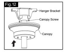
Slide the canopy up to ceiling and over the two screws on hanger bracket. Rotate canopy clockwise until tight.
