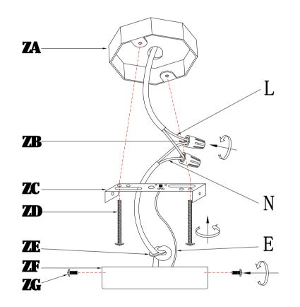
"L" = Hot wire "N" = Neutral wire "E" = Ground wire LDPD2021 D7"H5"L1
