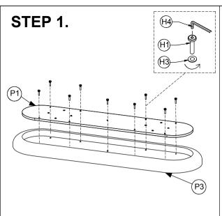
\*Screw the bolts out to take frame out (P1) of top (P3)
