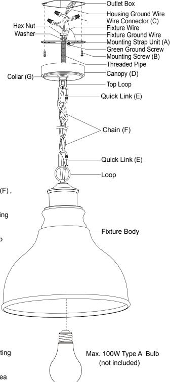
The following parts are available for re-order if damaged or missing.
