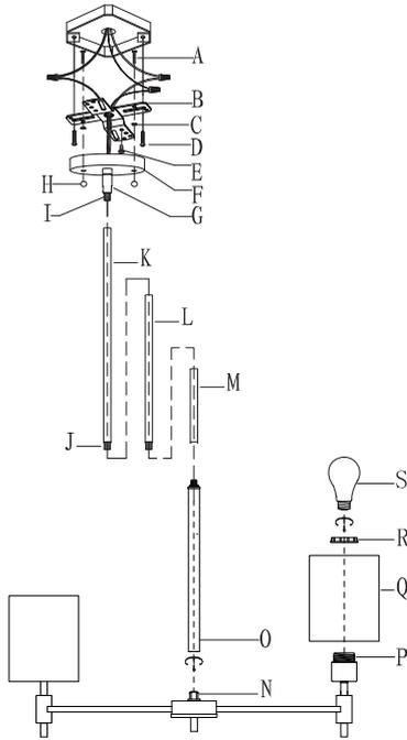
provided 6 inch rod (M) to hang the fixture. Thread the wires through the rods and pull the wires until taut before connecting the rods together. Screw bottom rod (M) onto rod (O). Screw the nipple of the top rod onto swivel post (I) of canopy (F). Pull the fixture wires through the top of the canopy.
