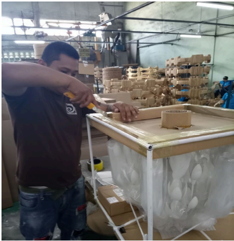
Step 4: Cut the Packaging tape Securing the top cardboard.
