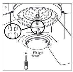
Connect white wire from fan to white wire from LED light fixture and then connect blue (or black) wire from fan to black (or blue) wire from LED light fixture.
