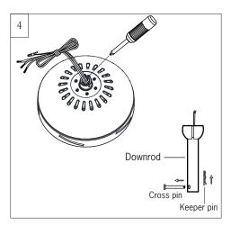
Partially loosen downrod set screws from yoke at top of motor assembly. Remove preassembled cross pin and keeper pin from downrod. Save parts.
