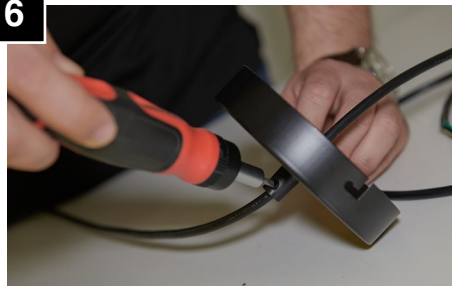
After adjusting cord length, tighten set screw on canopy.
