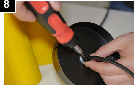
Slide down until it bottoms out and tighten set screw.
