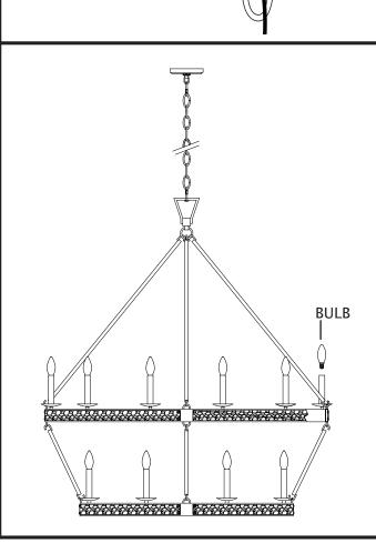
28. Screw recommended bulbs (E12 Candelabra bulb type, not included) into sockets. Verify correct bulb wattage marked on socket of fixture. **WARNING:** DO NOT exceed maximum bulb wattage
