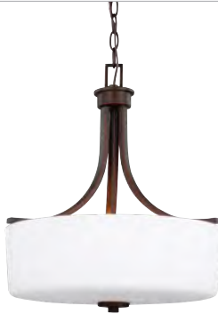
THREE LIGHT UPLIGHT PENDANT 6528803-710 D: 16" H: 18.5" Etched, White Inside Glass Socket: 100 W Medium T24 DAMP
