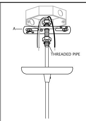
11. Slightly loosen ground screw on mounting bracket (A). Do not completely remove ground screw. Wrap house ground wire (copper) around ground screw, leaving enough ground wire to attach to fixture ground wire. Twist end of fixture ground wire and end of house ground wire (copper) together. Twist wire nut (C) onto ends of wires. Completely tighten wire nut (C). Reference chart below for correct wiring instructions.
