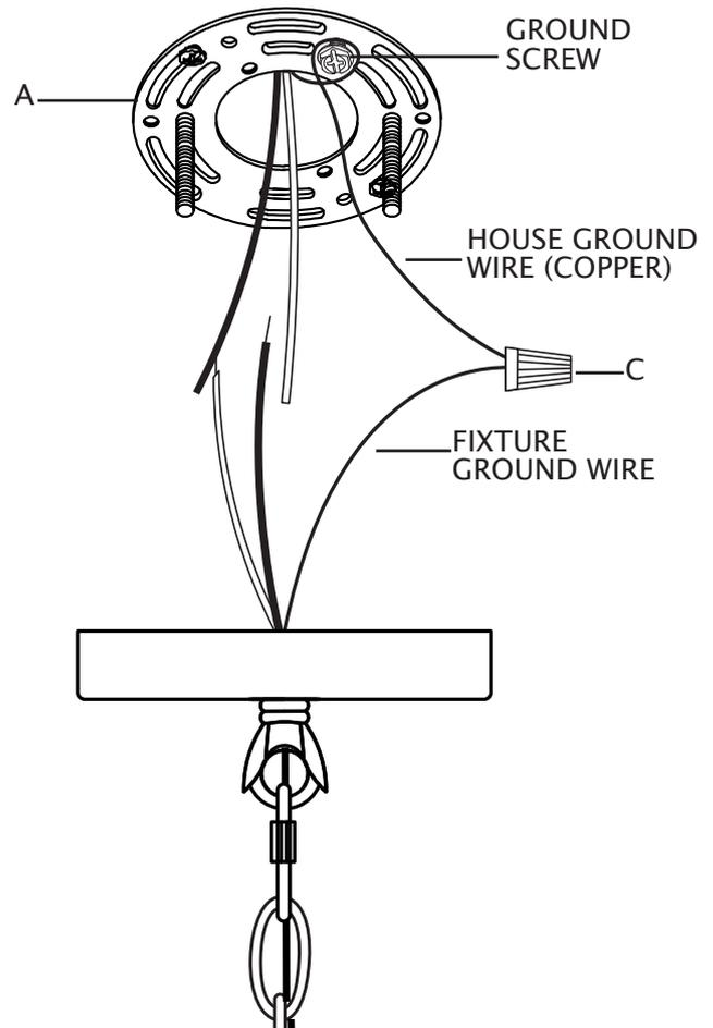
13. Twist end of house lead wire (black) and end of fixture lead wire together. Twist wire connector (C) onto ends of wires. Completely tighten wire connector (C). Twist end of house neutral wire (white) and end of fixture neutral wire together. Twist wire connector (C) onto ends of wires. Completely tighten wire connector (C). Reference chart to the right for correct wire connections.
