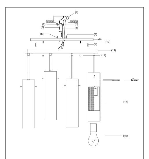
1.OUTLEX BOX 2.WIRE CONNECTOR 3. BLACK WIRE 4.WHITE WIRE 5.GROUND WIRE 6. BOX SCREW 7. WOOD SCREW 8. MOUNTING PLATE 9. GROUND SCREW 10. MOUNTING SCREW 11. CANOPY 12. BALL NUTS 13. BAR 14. SHADE 15. BULB
