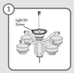
Remove the pre-installed light kit screws and replace them with the longer light kit screws provided.
