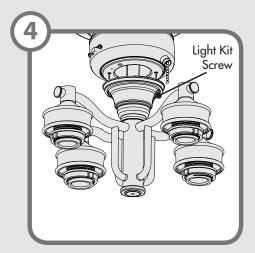
Lift the light kit up to meet the lower switch housing. Align the light kit screws with the threaded holes in the lower switch housing. Tighten screws securely.
