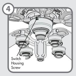
Lift the light kit assembly up so that the screw holes in the lower switch housing line up with the holes in the upper switch housing. Install the switch housing screws and tighten securely.
