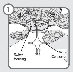
If your fan does not have pin connectors on the wires coming from the switch housing, install the wiring harness provided. Using the provided wire connectors connect the white wire from the fan to the white wire from the fan to the black or blue wire from the fan to the black wire from the wire harness.
